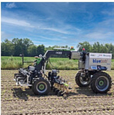
Six-row weeding with autonomously navigating field robot
