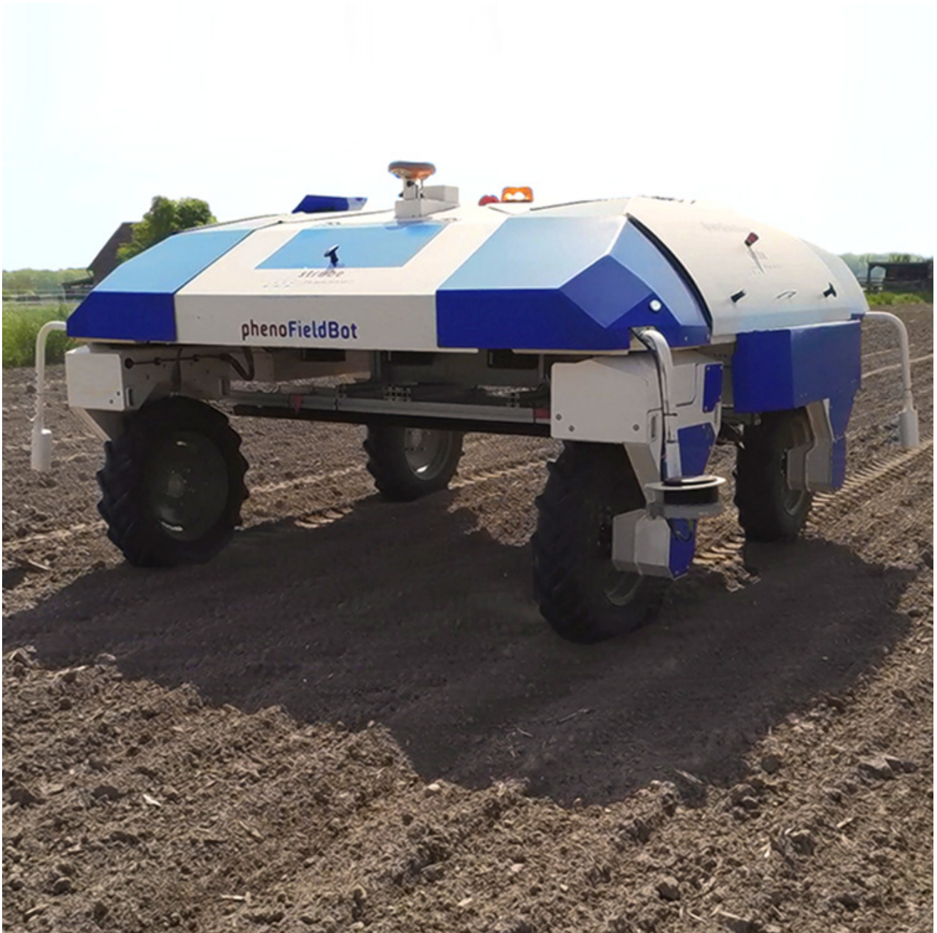
The phenoFieldBot starts already 11 days after sowing with the auton-omous measurement of the first plants.
