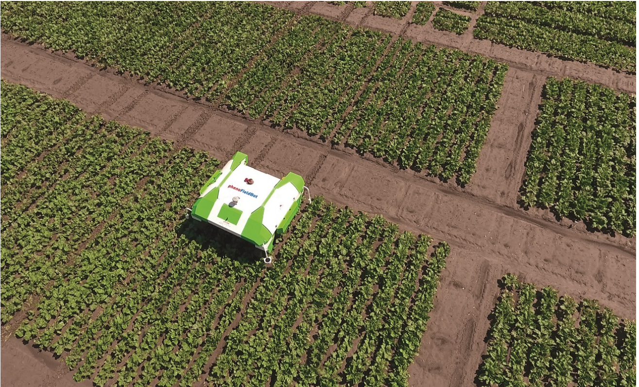
Strubes phenoFieldBot counts and measures plants.
